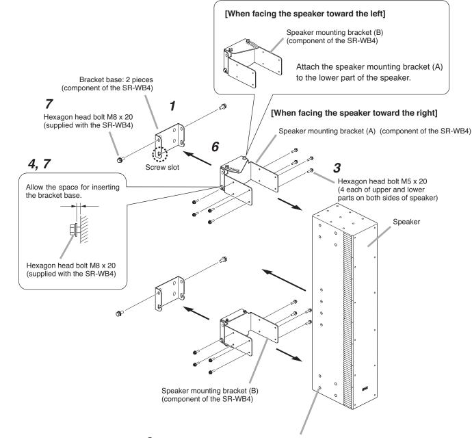
2 Remove the 16 attached screws (in upper and lower parts on both sides of speaker).
